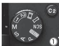
■ Aperture Priority Mode: Please set the camera mode dial to “A” (Aperture Priority) as shown in picture 2. Now the shutter speed will adjust when the aperture ring of the lens is rotated.
